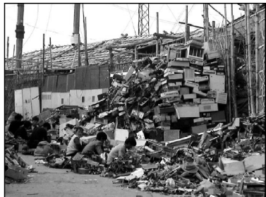
Very typical on-street E-waste dismantling operation in Guiyu. Using hammers and chisels and their bare hands, workers separate the waste into aluminum, steel, copper, plastic and circuit boards. © BAN
