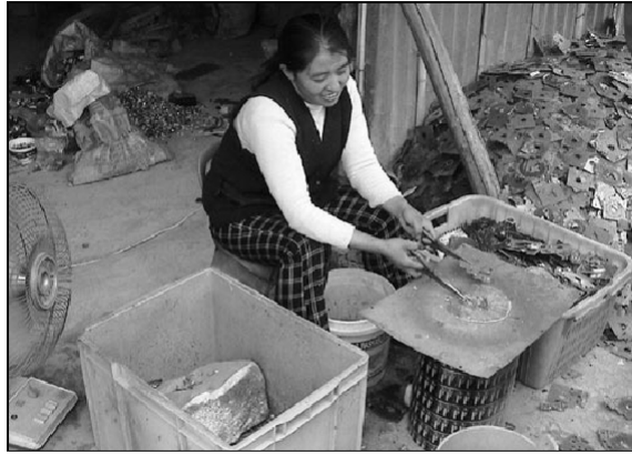
Laborer de-soldering circuit boards over a coal-fired grill. Rock in the box is where boards are hit to remove solder. Pliers are used to pluck off chips which go into various buckets. The boards are then tossed into a pile for open burning. © BAN
