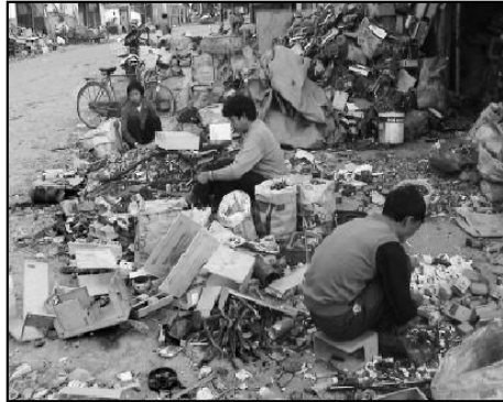
Typical E-Scrap operations in Guiyu, China. 100,000 such migrant workers labor in Guiyu breaking down imported computers in hundreds of small operations like this one in a 4 village area surrounding the Lianjiang River. Guiyu, China. December 2001. © BAN
